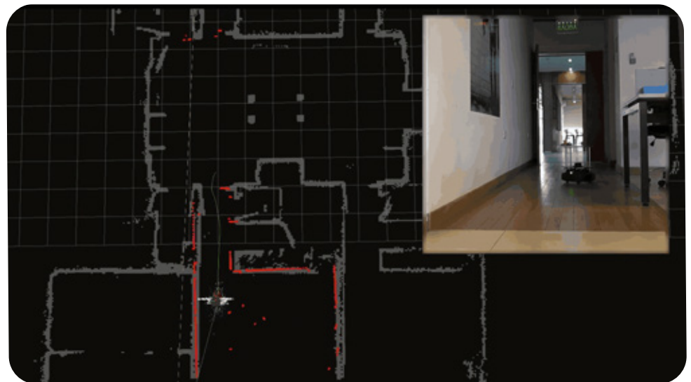
Beluga AMCL running on an Turtlebot 2 robot (Raspberry Pi 4B)
